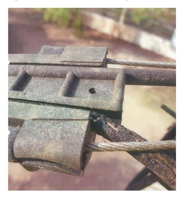
Figure 2. Showing degraded insulation and contact with steel braided cable
